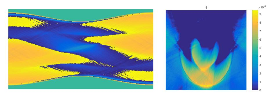
Tomographic reconstruction of wrapped phase data via the phase-SIRT algorithm
